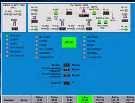
2. Temperature controlled Dryer
