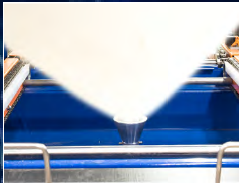
\ 2. \ Cloud dry developer applied (not actual powder in image)
