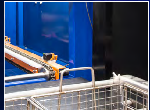
\ 3. \ Basket conveyed into unloading area
